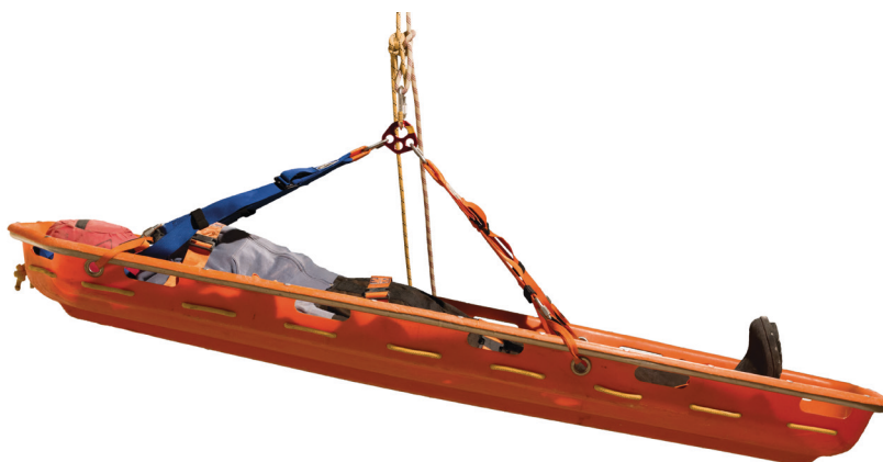
Figure 74: Casualty secured in a bucket stretcher, rigged horizontally and showing both the main and safety lines.
