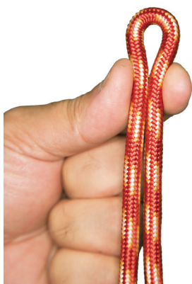
Figure 32: The pinch test is done to evaluate rope potential for use as Prusik rope. The inner diameter of the loop formed in the pinch test should be approximately equal to the outer diameter of the same cordage. 6 This ensures that the cordage is balanced in suppleness and stiffness to grab the rope sufficiently.
