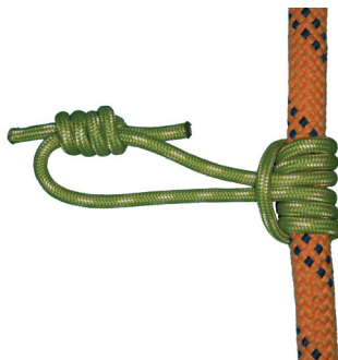
Figure 31: The Prusik hitch on a rope acts as a rope grab.
