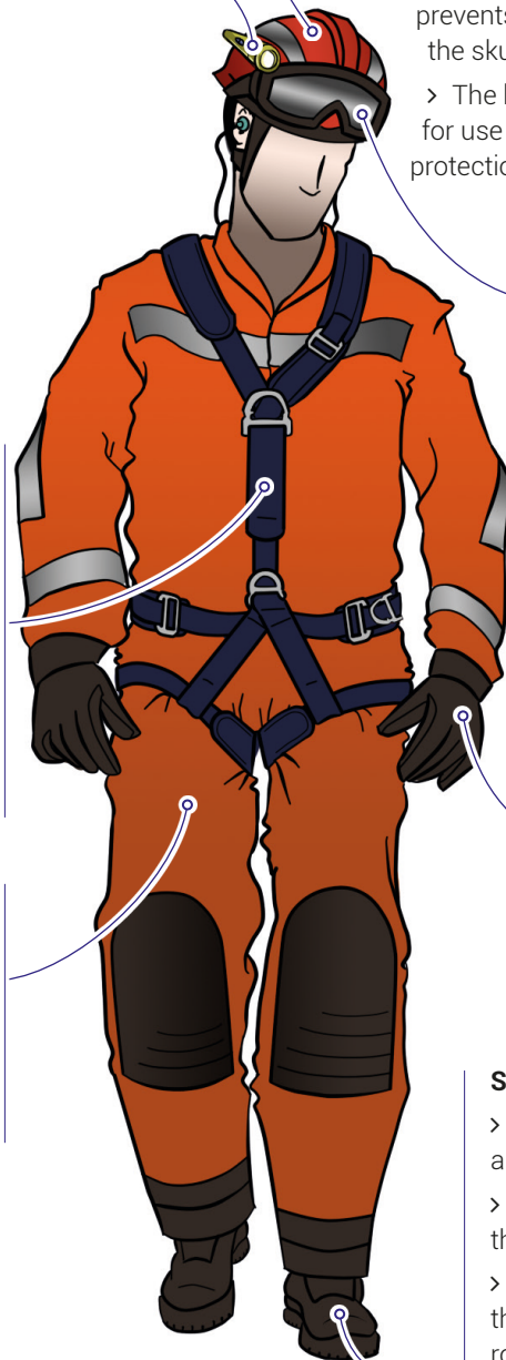
Figure 7: The rescuer with PPE appropriate to rope rescue operations. Key and recommended features of the different PPE parts are defined.
