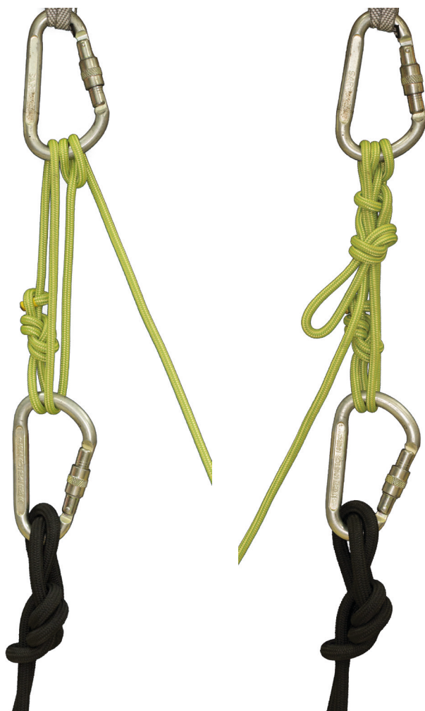
Figure 49: Radium release hitch.
