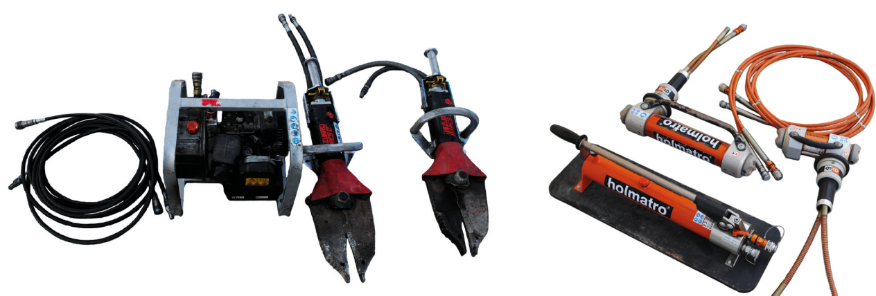
Figure 48: Hydraulic equipment – (a) hydraulic pump with hoses and cutters (b) hydraulic hand pump and rams.
