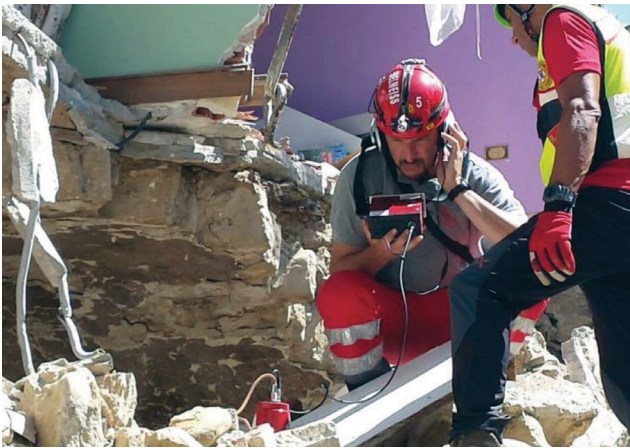
Figure 30a: A geophone in use at a collapsed building after an earthquake.
