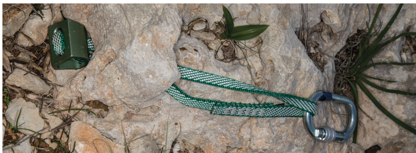
Figure 41: An anchor set on a rock outcrop using the hex system.
