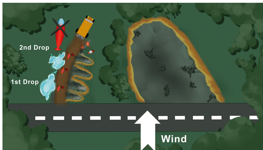
Figure 10: Combined tactics in indirect firefighting – a tractor creates a discontinuity, tactical fire is used to widen the discontinuity and aircraft drop water on unburnt fuel to prevent it from burning.
