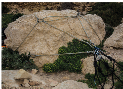
Figure 38: Boulder rigged anchorage.
