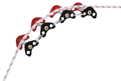
Figure 34: Edge protection in the form of mechanical protection whereby friction against abrasive terrain is avoided by rollers.
