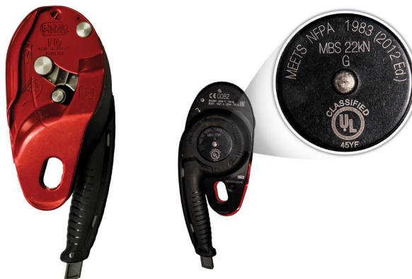
Figure 3: The image on the left shows the front side of a Petzl I'D L descender while the image on the right shows the back part of the same I'D version with its magnified central part. The NFPA markings (being the 'L' version), show a notation 'G' indicative of general use, hence able to withstand larger forces than the equivalent 'T' equipment.
