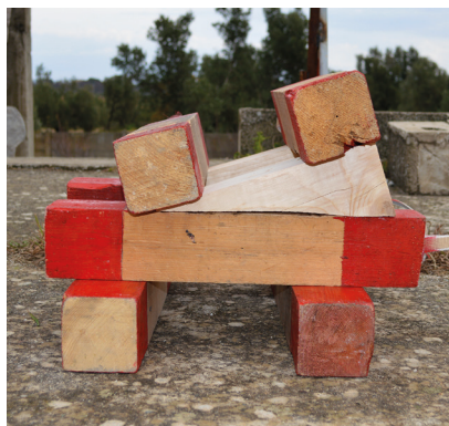
Figure 44: (a) Example of wedges on top of box cribbing. (b) Supporting a slanting load with box cribbing and wedges.
