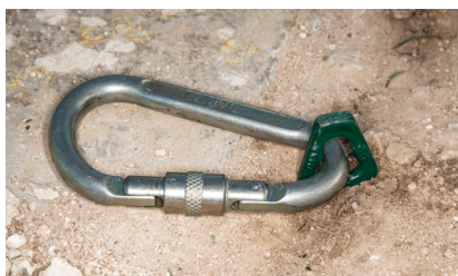
Figure 42: Piton embedded in compact soil with carabiner in eyelet for sling or rope attachment.
