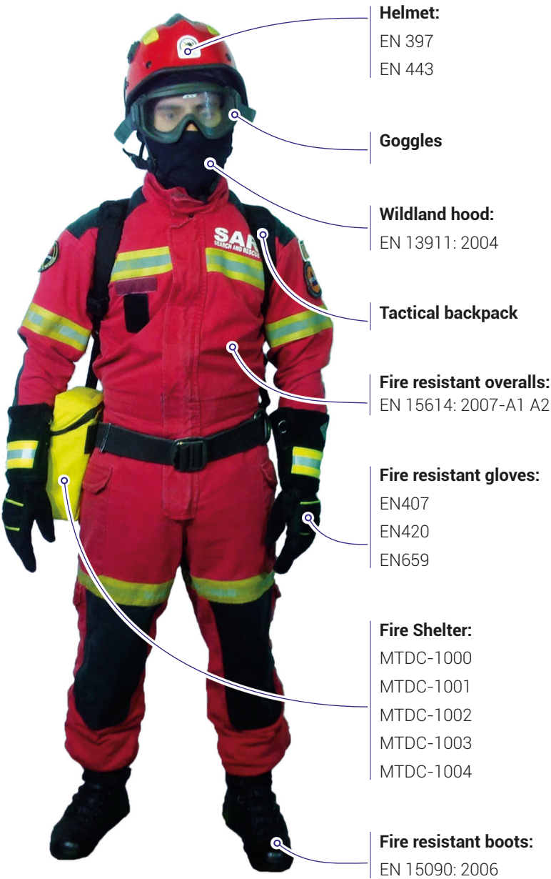
Figure 12: Typical PPE used by firefighters in wildfire response and applicable standards
