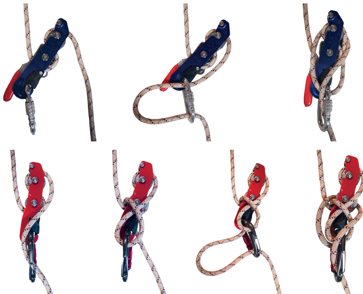
Figure 35: Sequence for locking (a) the Petzl STOP and (b) the Petzl SIMPLE.
